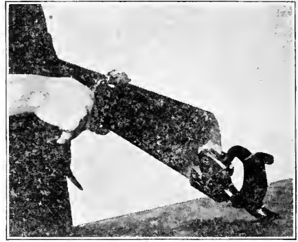
FIG. 110. SETTING SAW TEETH.
